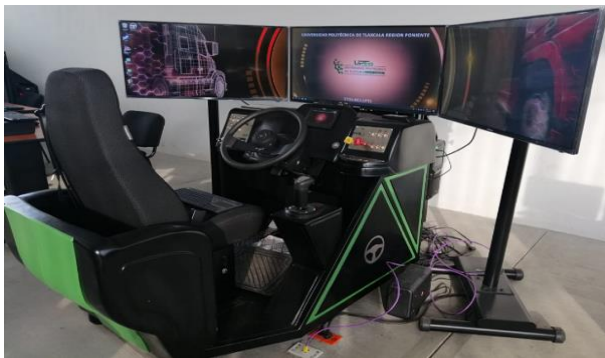
Figure 1 Driving Simulator Big Rig 2 HD Source: Engineering in Logistics and Transportation . UPTrep
